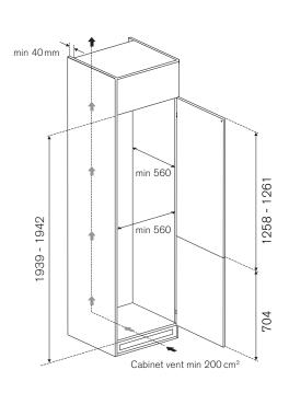
The refrigerator is installed on the cabinet base shelf and not on the kitchen floor.
